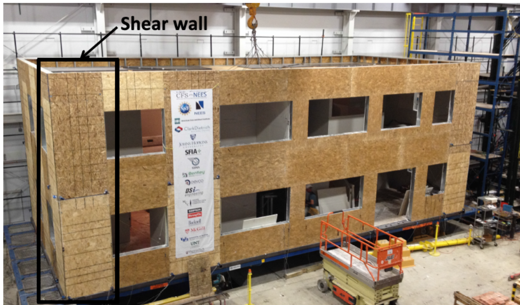
Figure 6-1. CFS-NEES building and shear wall in it
